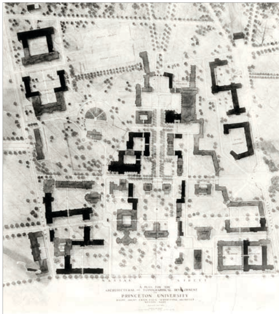
Plan for the Architectural and Topographical Development of Princeton University, Ralph Adams Cram, 1911 This plan reveals a subtle combination of axial symmetry with informal building arrangements following the terrain. New buildings define courtyards and create walls around the edge of campus, separating it from the surrounding town. A notable feature of the plan is its 'upside down' orientation—with north pointing downwards—so that Nassau Hall is clearly identified as the front of campus.
