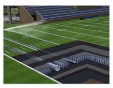
Under-Field Storage, Subsurface Infiltration and Green Roofs
